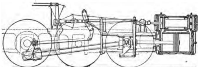
FIG. 11.—Piston Valve Actuated by Walschaert Gear.
