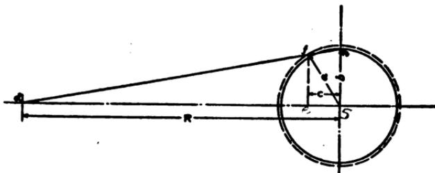
FIG. 31.—Laying-out Diagram, Walschaert Valve Gear.
