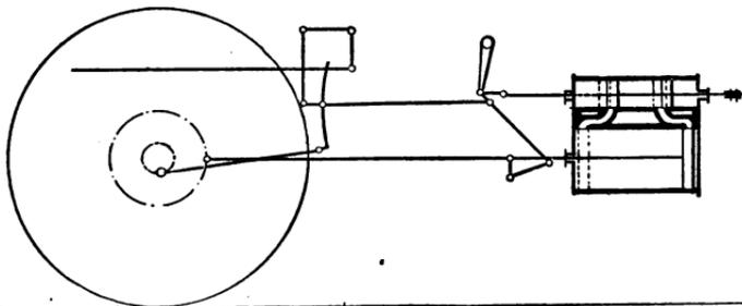
FIG. 24.—Side Elevation Diagram of Belgian Engine.
