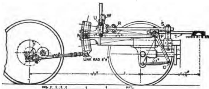
FIG. 10.—Mason's Improved Design of Walschaert's Valve Gear.
