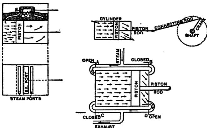
FIG. 1.—The Main Valve; showing admission and exhaust ports, the cylinder and piston.
