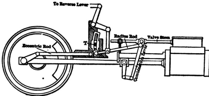
FIG. 6.—Building up the Walschaert Valve Gear.
